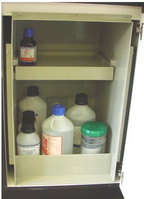
**Figure 4 – Bottles stored in drip trays within ventilated acids cabinet including example of chemically resistant secondary containment (BDH / VWR Safepak bottom right)**
