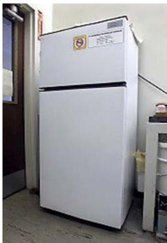
**Figure 1 – modified domestic-type refrigerator used to store chemicals**
