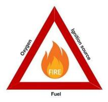
In the above diagram the fuel is the hazardous substance such as petrol, solvent, paint thinners etc.
